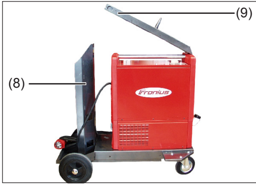
Fig.20 Mount the wirefeeder fixture
