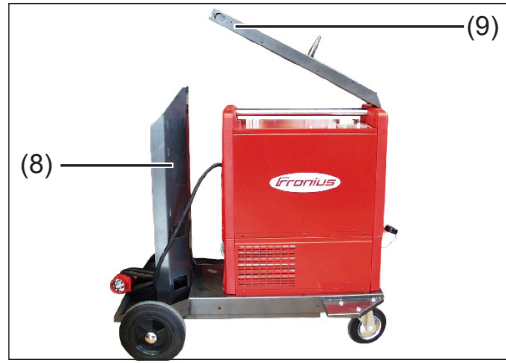
Fig.13 Dismount the wirefeeder fixture
